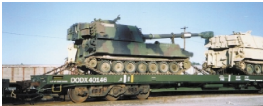
Pilot model of 150 ton flat car (un-painted) shown with production versions of M992 and Paladin.
